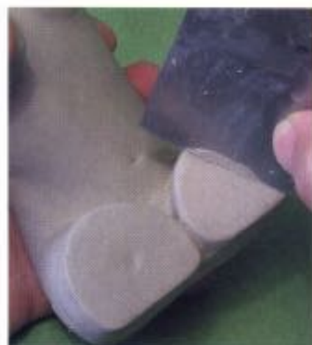
Use a flat paint scraper to refine the joining surfaces.
